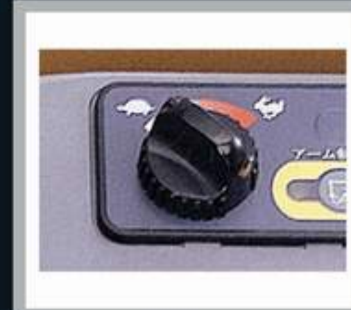
Rotary Engine Throttle with Auto Idling System
